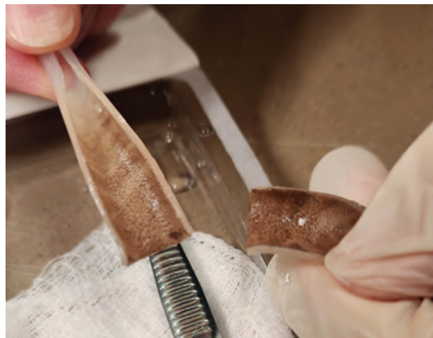
Picture 1: Bisected transfer set with brown discoloration
